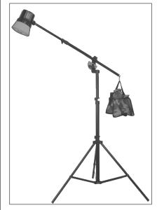
Attach light head on spigot Raise central coloum to desired height.
