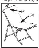
top edge (A) under the locking brackets. Then press down at the center of the sheet (B) to enable the lower edge (C) to slide into the locking brackets easily.(The matte surface should stay on the top)
